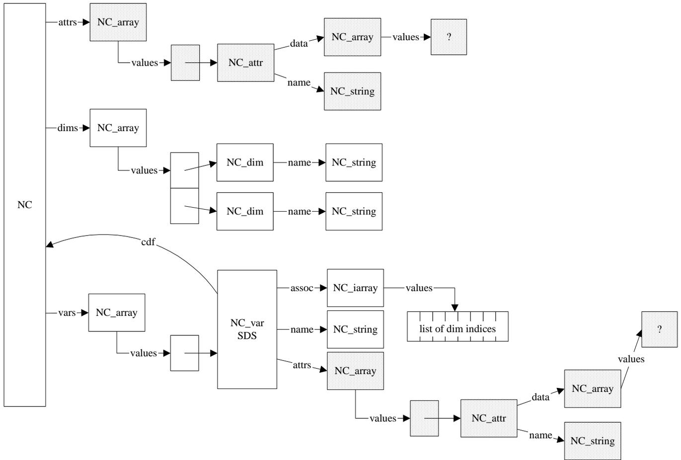
FIGURE 7x SD collection contents in memory after adding a dimension attribute
