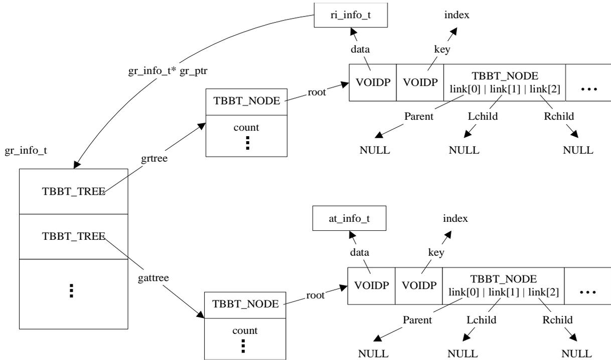
FIGURE 8r **Illustration of data structure ri\_info\_t**
