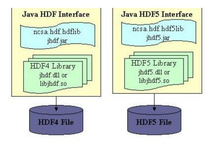
The native code will need to build the libraries (including dependent external libraries) and the interface test. Finally all the libraries will need to be packaged on all the standard platforms that HDF supports, Windows, OS X, and Linux. The release process has one target; just the platform native libraries.
