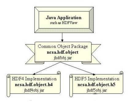
The HDFView and object model build and test process will need to include the native package for the platform under test. The release process has one target; the HDFView and class jar files with platform native libraries. These jar files will be packaged on all the standard platforms that HDF supports, Windows, OS X, and Linux with a current version of Java. In addition, each distribution will include a JRE.
